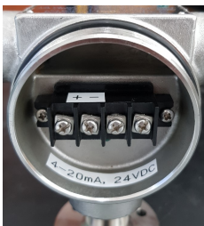
ZT-100 Wiring Terminal (2 wire loop powered)
